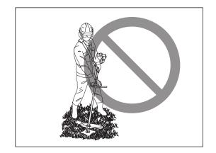
Do not operate with holding the brush cutter at the higher position than your waist.
