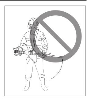
Do not operate while you are moving backward. You could trip over and fall down, resulting in unexpected injury.
