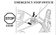
Press the emergency stop switch to stop the engine.
