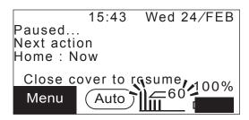
Check that the setting value (20 – 60) of the cutting height is selected and press the button.
