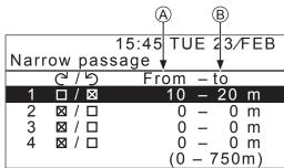
B: Distance between the docking station and the end of the narrow passage.
