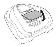
Press the manual STOP button. The control panel cover pops up.
