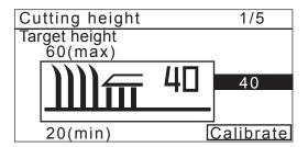
Set the "Start cutting height" with the ♠ ♥ buttons or number buttons and press the 🕘 button.
