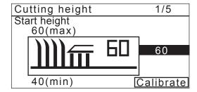
When you select [Calibrate] and press the e button, the blade disc moves to the set cutting height. You can check the cutting height.
