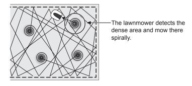
With this function, you can concentrate the lawnmower on mowing the dense area of lawn during the normal operation.
