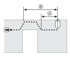
(A): Distance between the docking station and the start of the narrow passage.
