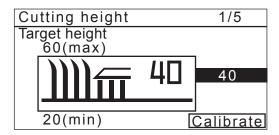
3 Set the "Start cutting height" with the 🌢 👽 buttons and press the 🕘 button.
