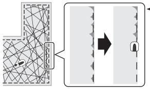
If the edge cutting setting is enabled, the lawnmower goes around your garden along the boundary wire to mow the edge before starting the usual mowing.
