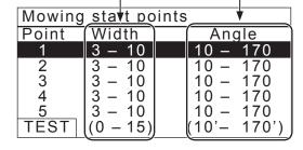
When leaving the boundary wire, set the minimum and maximum angle to turn from the boundary wire.
