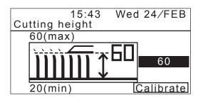
Set the cutting height with the A  $\textcircled{\P}$  buttons and press the e button.
