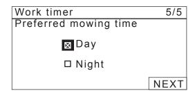
Confirm the days which are automatically selected referring to the boundary wire length and garden size. Select [NEXT] and press the button to proceed to the timer setting screen.
