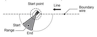
TIPS Use the exit angle to let the lawnmower reach the mowing areas directly instead of using long wire exit locations.
