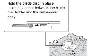
Replace the blades, insert each blade through each bolt on the blade disc, and lightly tighten a nut with the 8 mm spanner.
